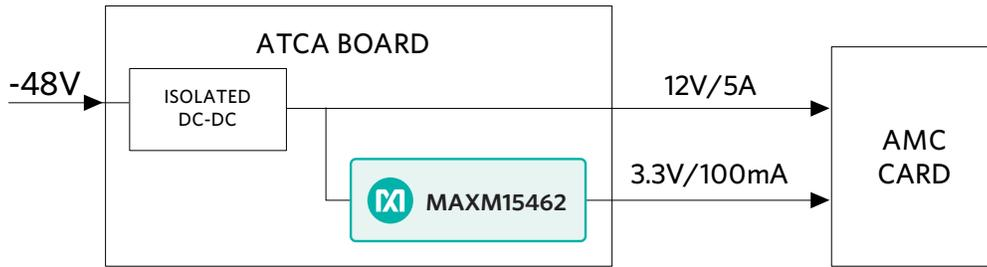
Figure 11. An ATCA board powering an AMC card
