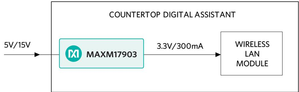
Figure 13. MAXM17903 uSLIC powering wireless LAN module
