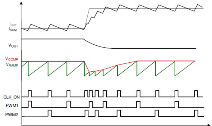
Figure 1 Load insertion response
