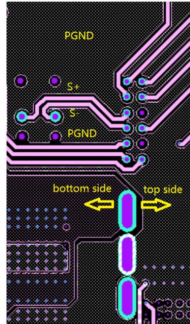
**Figure 3 sense+/- layout example**
