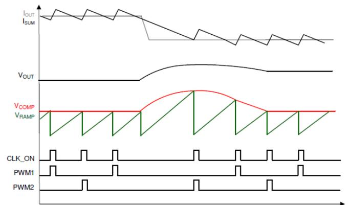
Figure 2 Load release response
