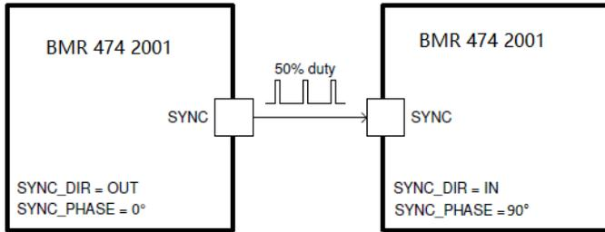
**Clock master module drive a clock slave module**
