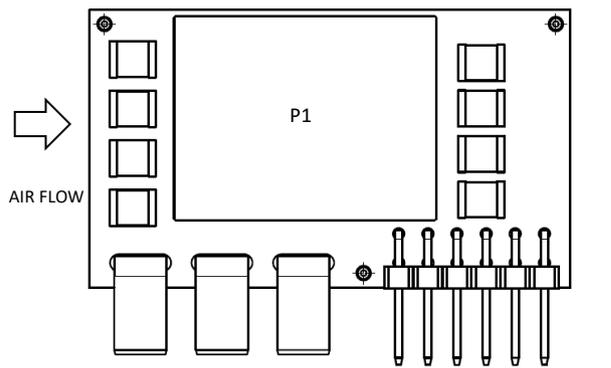
Temperature positions and air flow direction (top side view)
