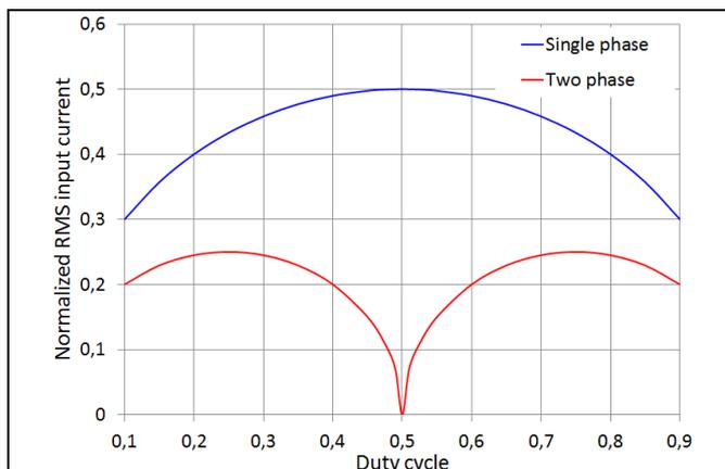
The input ripple RMS current in a buck converter can be estimated to
