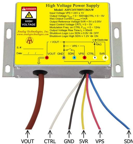
Figure 2. The Connecting Lead Wires of AHV24V500V1MAW
