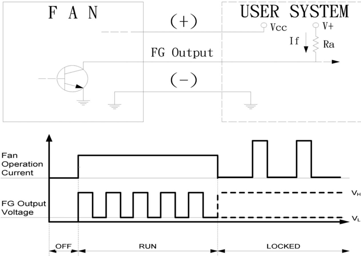
★Electrical Characteristics : ( at  $T_a = 25^\circ\text{C}$ ,  $V_{CC}=5\text{V}$ )
