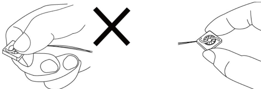
**Don't pull fan with lead wires.**
