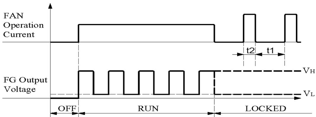
★Electrical Characteristics : ( at Ta = 25°C ) Vcc = 5V±10%
