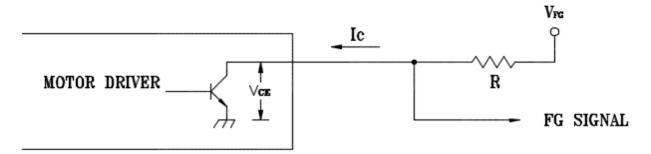
CAUTION: THE LEAD WIRE OF FG SIGNAL CAN NOT TOUCH THE LEAD WIRE OF POSITIVE OR NEGATIVE
