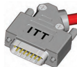
Assemble the other half (screwing force: 100-120 Ncm)
