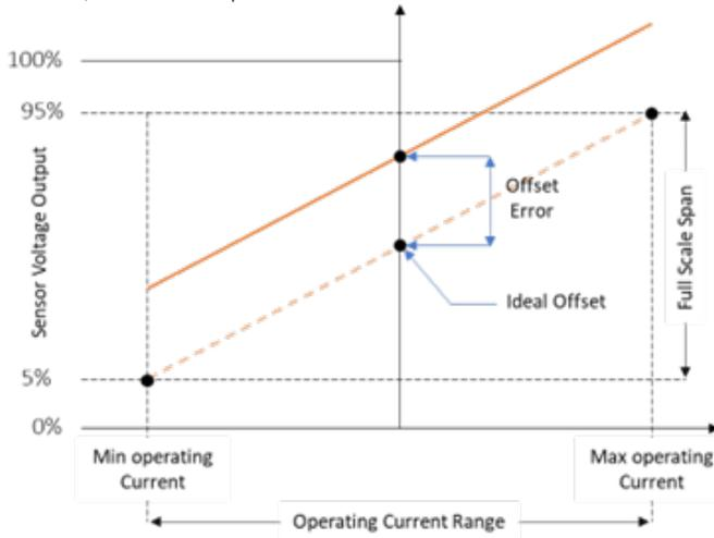
Figure 2: Exaggerated Offset Error.
