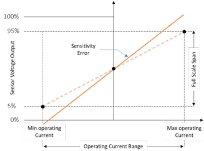
Figure 3: Exaggerated Gain Error
