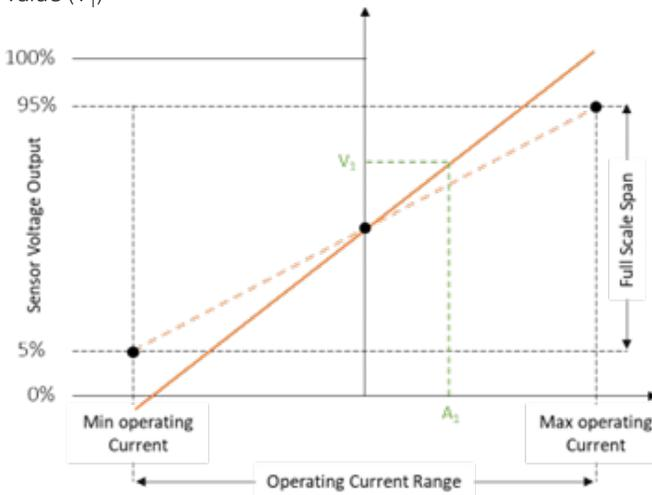
Figure 5: Simple Gain Calibration
