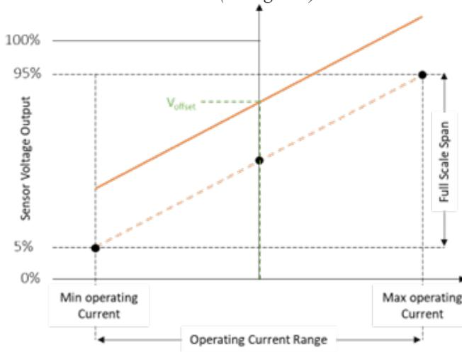
Figure 4: Simple Offset Calibration
