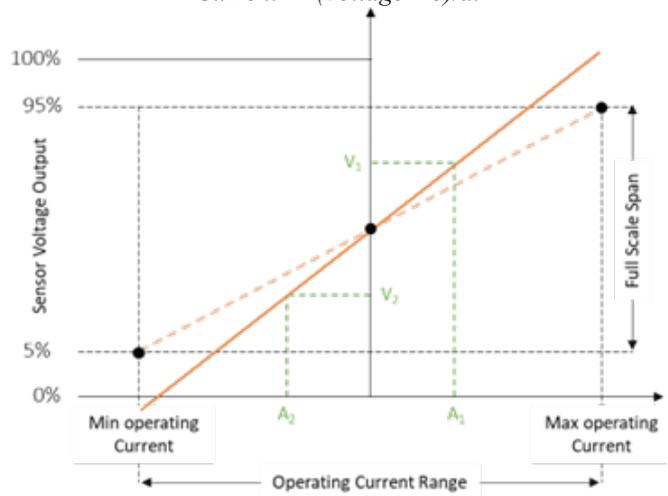
Figure 6: Gain Calibration
