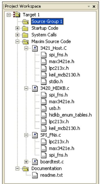
Figure 8. Structure of the Keil Project.
