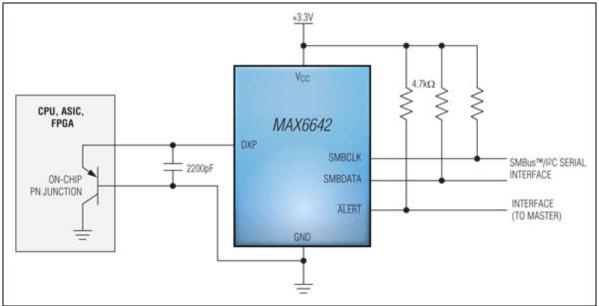
Figure 4. A remote temperature sensor, the MAX6642, monitors the temperature of a sensing transistor (or thermal diode) on the die of an external IC.
