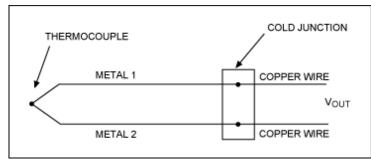
Figure 2. Simple thermocouple circuit. The junction between metal 1 and metal 2 is the main thermocouple junction. Other thermocouples are present where the metal 1 and metal 2 wires join with
