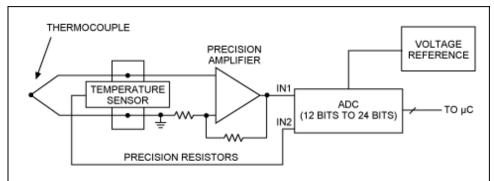
Figure 3. Example of a thermocouple signal-conditioning circuit.
