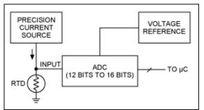
Figure 1. Simplified RTD signal-conditioning circuit.
