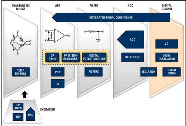
Block diagram of the signal chain in a force-sense application. For a list of Maxim's recommended pressure-sensor solutions, please go to: www.maximintegrated.com/psi.
