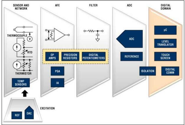
Block diagram of the signal chain in a temperature-sensing application. For a list of Maxim's recommended temperature-sensor solutions, please go to: www.maximintegrated.com/-40+85.
