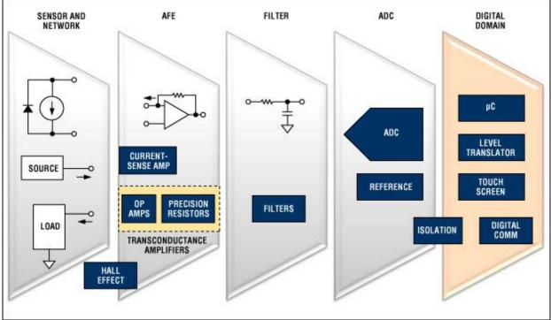
Block diagram of the signal chain in a current-sensing application. For a list of Maxim's recommended current-sensing solutions, please go to: www.maximintegrated.com/detect.
