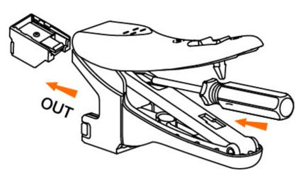
Use the slotted screwdriver to push out the cutting module as shown
