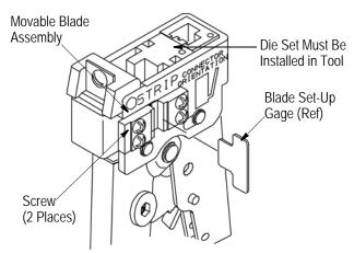
**CAUTION:** DO NOT cycle the tool without the die set in place; otherwise, damage to the stripping blades may occur.
