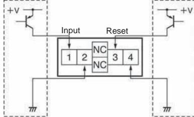
or Open collector of an NPN transistor
