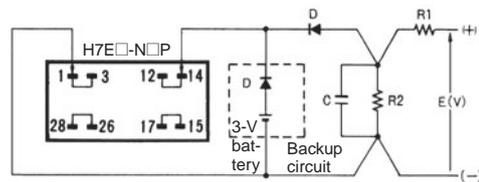
Use a diode (D) having a forward voltage as small as possible (0.1 V max. at I<sub>F</sub> of 20 μA).
