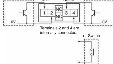
Terminals 2 and 4 are internally connected.
