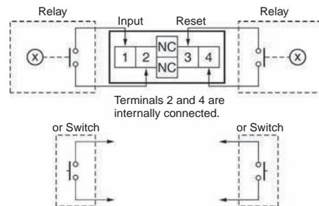
Terminals 2 and 4 are internally connected.
