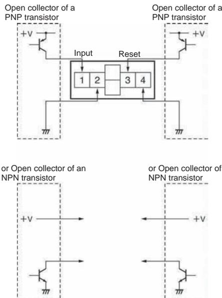
**Note:** 1. Terminals 2 and 4 (input circuit and reset circuit) are functionally isolated.
