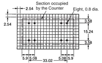
Note: Processing dimensions are for 28-pin IC socket.
