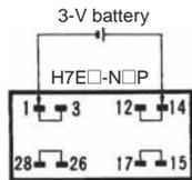
When designing a circuit, keep the power wiring connections shorter than 50 mm. Refer to the connection diagram above for the proper wiring polarity.
