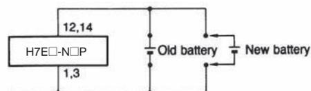
Wiring polarity must be carefully observed, in order to prevent permanent damage to the Counters. Exercise caution when inserting the Counter in the socket, to prevent reversed polarity.
