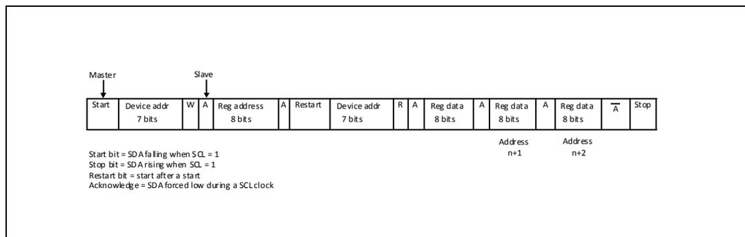
Figure 5. Write operation
