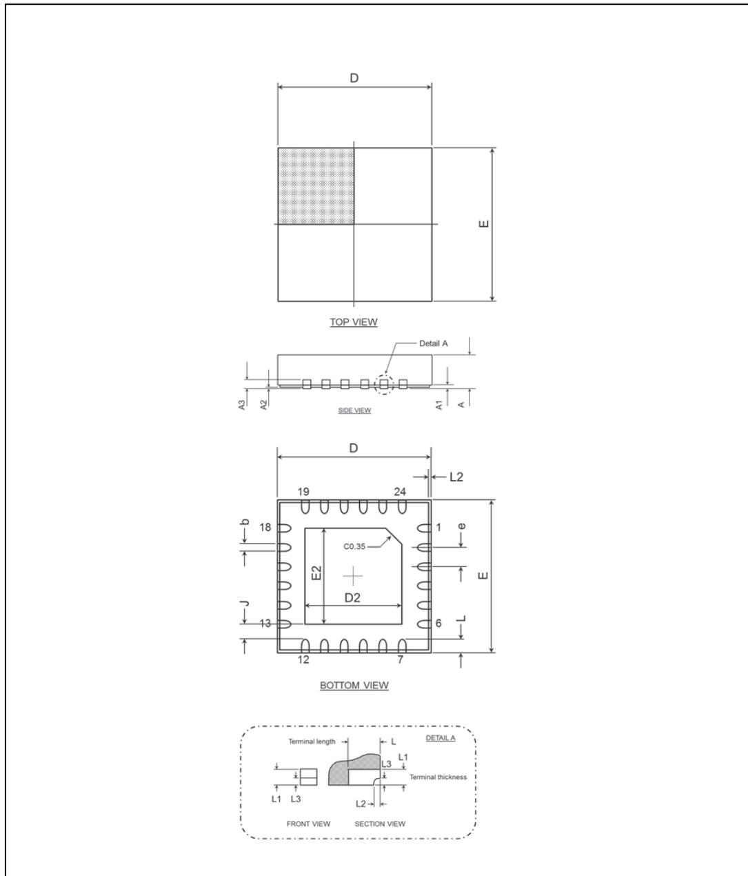
Table 40. QFN24 EP 4x4 Wet Flk mm mechanical data
