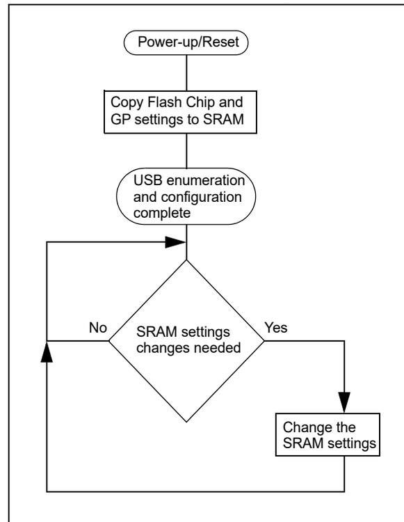
The SRAM settings (GP and partial Chip settings) can be modified through USB HID commands, and they will have an effect on the following device features:
