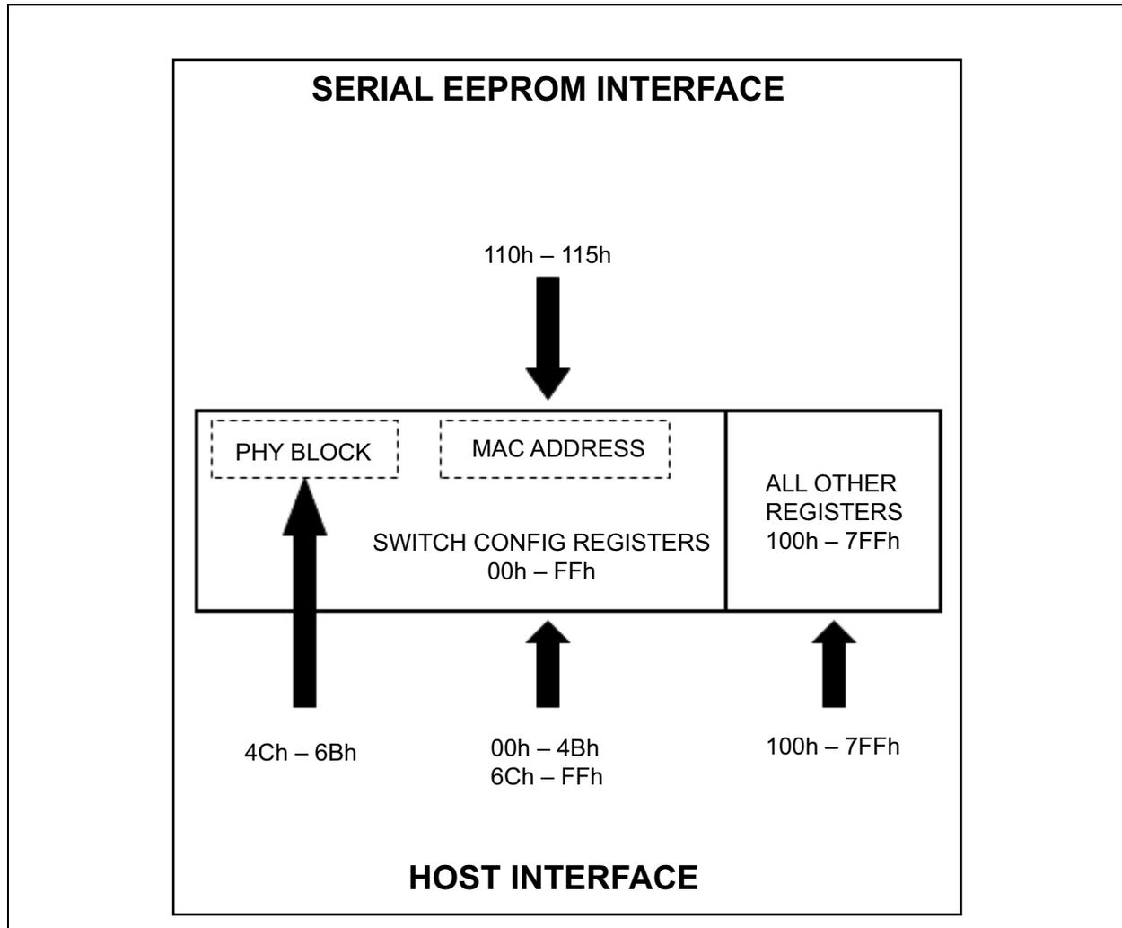
The registers within the linear 0x000 – 0x7FF address space are all accessible via the host interface bus by a microprocessor or CPU. The mapping of the various functions within that linear address space is summarized in [Table 4-1](#).
