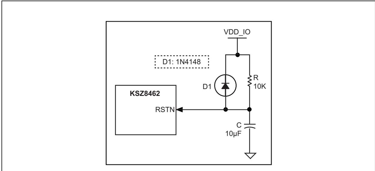
The following reset circuit is recommended for applications where reset is driven by another device (e.g., CPU or FPGA). At POR, R, C, and D1 provide the necessary ramp rise time to reset the KSZ8462 device. The RST\_OUT\_N from CPU/FPGA provides the warm reset after power-up.
