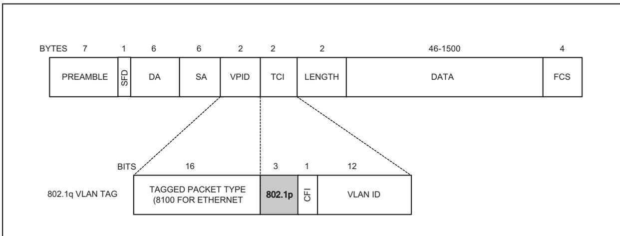
802.1p-based priority is enabled by bit[5] of registers P1CR1, P2CR1, and P3CR1 for ports 1, 2, and the host port, respectively.
