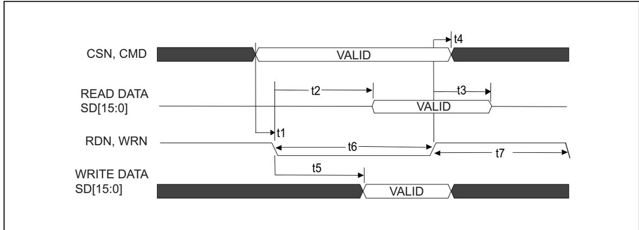
**TABLE 7-1: HOST INTERFACE READ/WRITE TIMING PARAMETERS**
