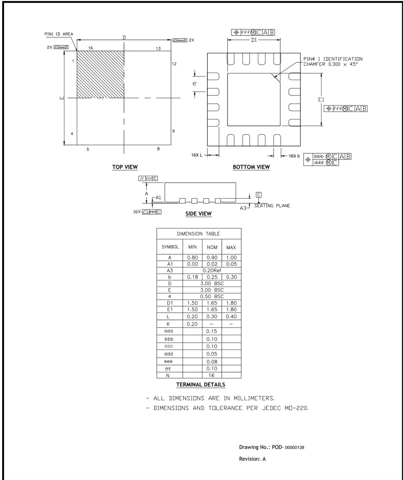
**NOTE:** QFN16 3x3  $\theta_{JA} = 36.4^{\circ}\text{C/W}$ ,  $\theta_{JC} = 17.8^{\circ}\text{C/W}$ . All values are typical.
