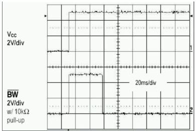
Figure 2. Power-on battery test fails ( $V_{BAT} = 2.55V$ ).
