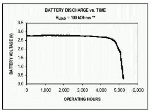
Figure 1. Battery discharge plot.
