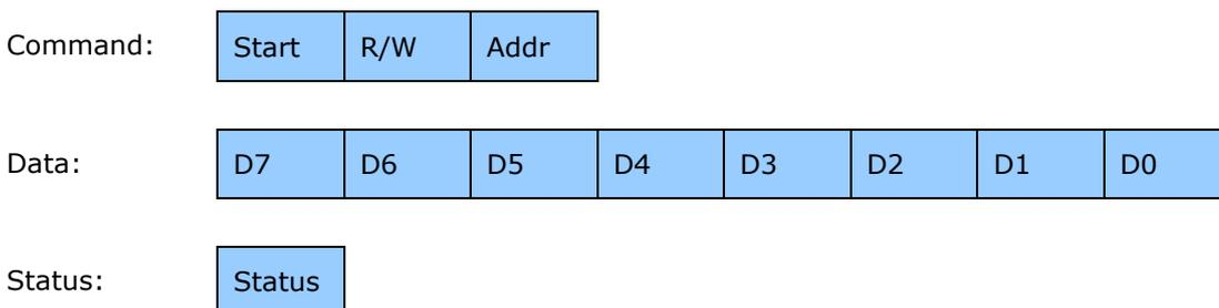
**Figure 6.15 VNC1L Compatible SPI Command and Status Structure**
