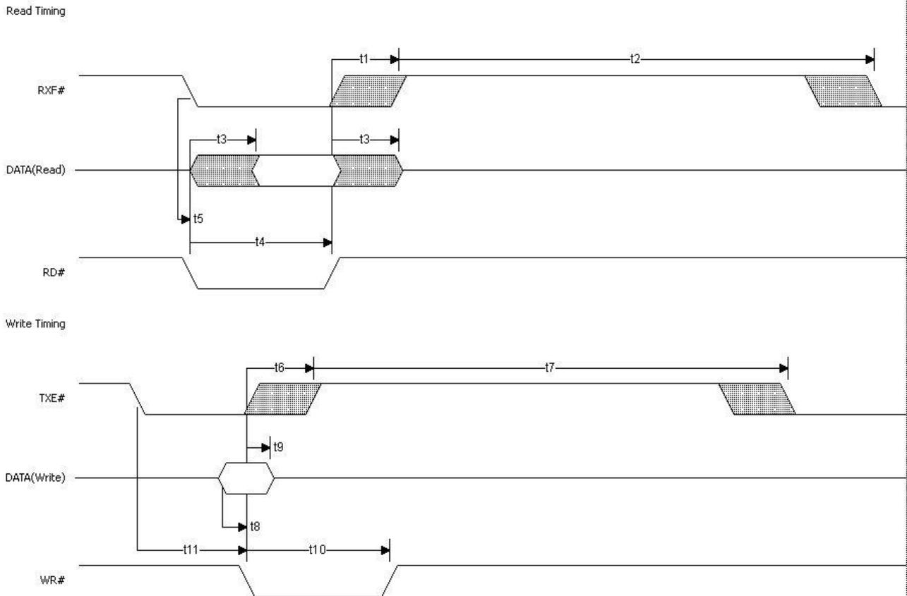
**Figure 6.22 Asynchronous FIFO mode Read / Write Cycle**
