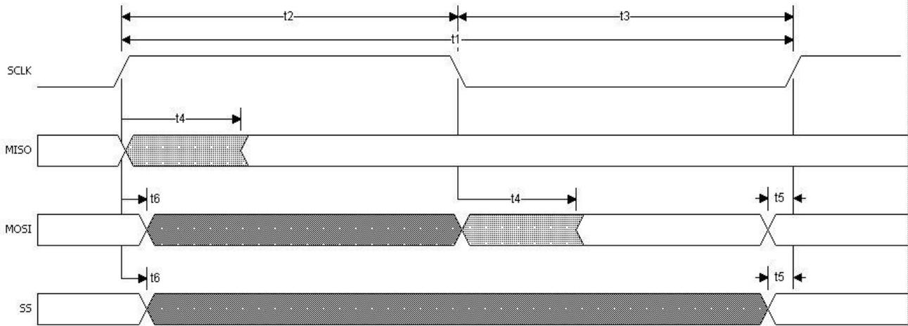
**Figure 6.16 SPI Slave Mode Timing**
