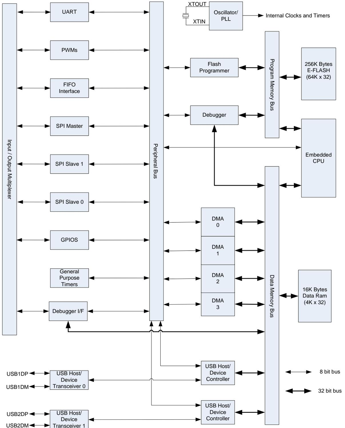
Figure 2.1 Simplified VNC2 Block Diagram
