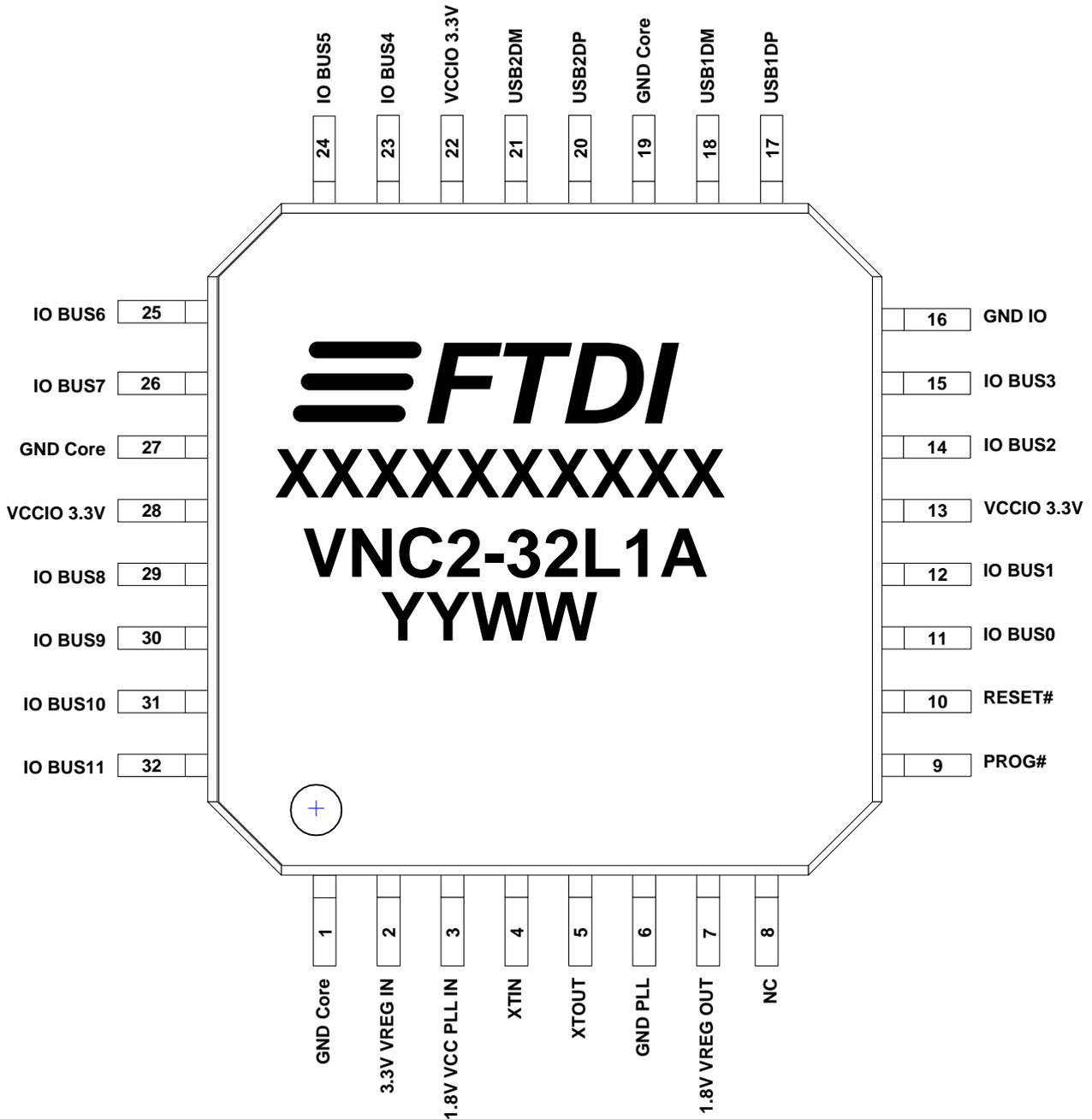
**Figure 3.1 32 Pin LQFP – Top Down View**
