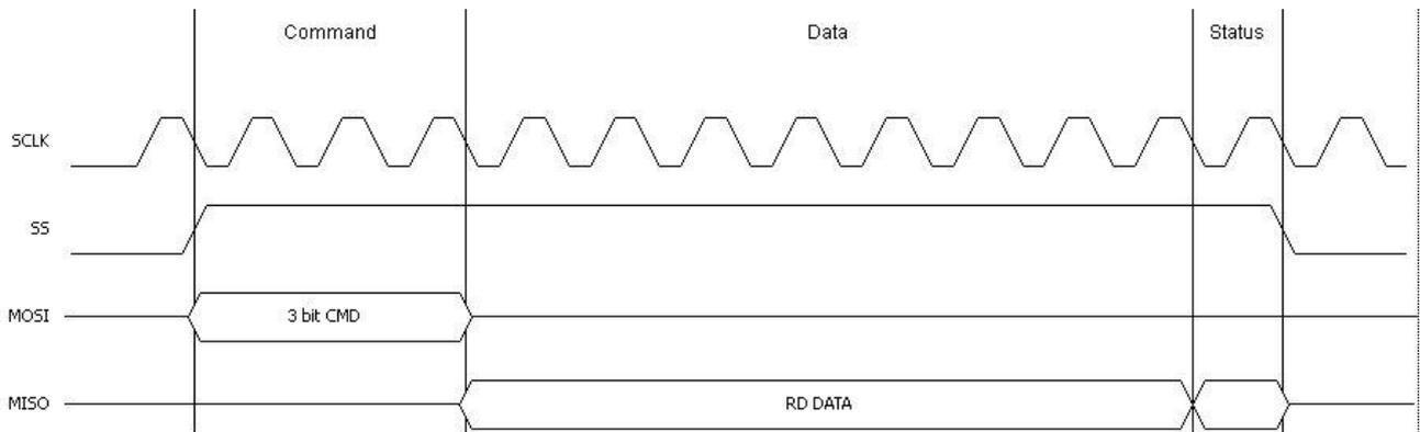
**Figure 6.17 SPI Master Data Read (VNC2 Slave Mode)**
