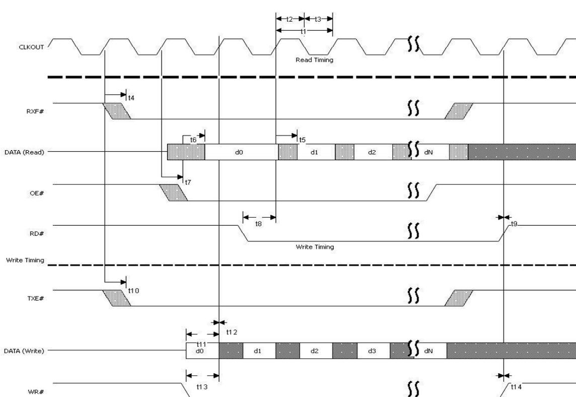
**Figure 6.23 Synchronous FIFO mode Read / Write Cycle**
