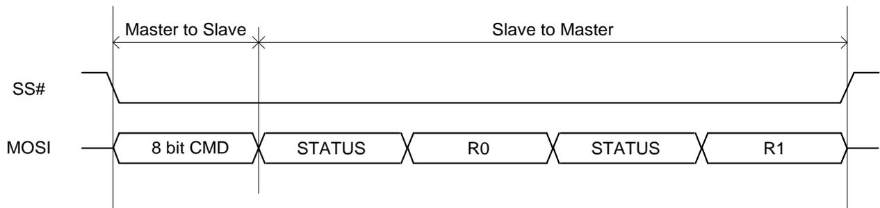
**Figure 6.11 Half Duplex 3-pin Data Master Read**
