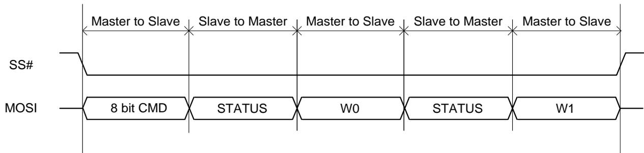
**Figure 6.10 Half Duplex 3-pin Data Master Write**
