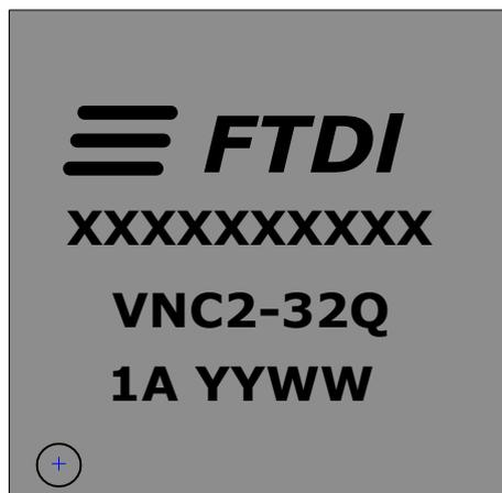
**Figure 11.2 Markings – 32 QFN**
