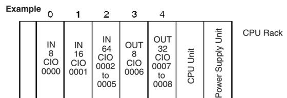
**2. Allocations to CS1 Expansion and C200H Expansion I/O Racks**
