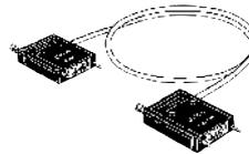
These cables are used to connect a CPU Unit to an Expansion I/O Rack, or to connect two Expansion I/O Racks. Select cables from among the following five types, and use them in combination when necessary. The total cable length must be within 12 m.
