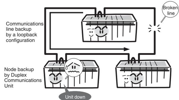
**Note:** The CS1W-CLK12-V1 or CS1W-CLK52-V1 is required for network duplexing.
