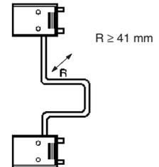
CS1 to C200H I/O Connecting Cable (Cable diameter: 5.1 mm)
