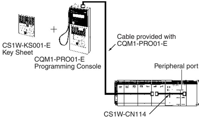
**Note:** The above configuration is also possible for the C200H-PRO27-E with a Programming Console Cable, such as the C200H-CN222.
