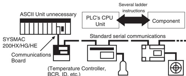
**Note:** An optional Communications Board (C200HW-COM04-E/05-E/06-EV1) is required to use the Protocol Macro function.
