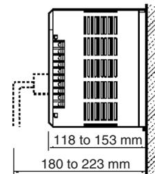
**Note:** I/O Connecting Cables require sufficient space to maintain the min. bending radius.
