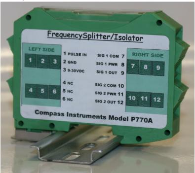
The Compass Instruments P770A Frequency Splitter/Isolator may be used to create two identical isolated frequency outputs from one frequency/pulse input.
