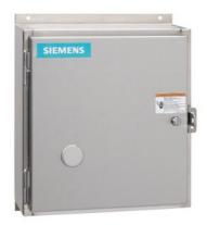
Electrically held lighting contactor, Contactor amp rating 30A, 0 N.C. / 4 N.O. Poles, 347VAC 60HZ coil, Non-combination type, (no disconnect device), Encl NEMA type 4X 304 S-Steel, Water/dust tight noncorrosive
