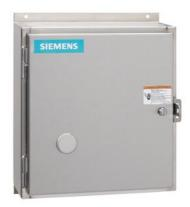
Electrically held lighting contactor, Contactor amp rating 30A, 0 N.C. / 3 N.O. Poles, 600VAC 60HZ coil, Non-combination type, (no disconnect device), Encl NEMA type 4X 304 S-Steel, Water/dust tight noncorrosive
