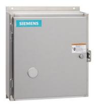
Electrically held lighting contactor, Contactor amp rating 30A, 0 N.C. / 3 N.O. Poles, 480VAC 60HZ coil, Non-combination type, (no disconnect device), Encl NEMA type 4X 304 S-Steel, Water/dust tight noncorrosive
