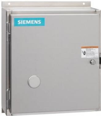
Electrically held lighting contactor, Contactor amp rating 20A, 0 N.C. / 3 N.O. Poles, 480VAC 60HZ coil, Non-combination type, (no disconnect device), Encl NEMA type 4X 304 S-Steel, Water/dust tight noncorrosive
