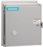
Electrically held lighting contactor, Contactor amp rating 20A, 0 N.C. / 3 N.O. Poles, 220VAC 50HZ/240VAC 60HZ coil, Non-combination type, (no disconnect device), Encl NEMA type 4X 304 S-Steel, Water/dust tight noncorrosive
