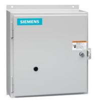
Electrically held lighting contactor, Contactor amp rating 30A, 0 N.C. / 4 N.O. Poles, 198VAC 50HZ/208VAC 60HZ coil, Non-combination type, (no disconnect device), Enclosure NEMA type 12, Dust/drip proof for indoors
