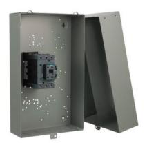
Electrically held lighting contactor, Contactor amp rating 100A, 0 N.C. / 3 N.O. Poles, 277VAC 60HZ coil, 1 NO / 1 NC auxiliary contacts Non-combination type, (no disconnect device), Enclosure NEMA type 1, Indoor general purpose use
