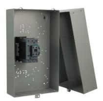
Electrically held lighting contactor, Contactor amp rating 100A, 0 N.C. / 3 N.O. Poles, 24VAC 50/60HZ coil, 1 NO / 1 NC auxiliary contacts Non-combination type, (no disconnect device), Enclosure NEMA type 1, Indoor general purpose use
