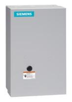
Electrically held lighting contactor, Contactor amp rating 30A, 0 N.C. / 6 N.O. Poles, 110VAC 50HZ/120VAC 60HZ coil, Non-combination type, (no disconnect device), Enclosure NEMA type 1, Indoor general purpose use
