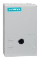
Electrically held lighting contactor, Contactor amp rating 30A, 0 N.C. / 3 N.O. Poles, 480VAC 60HZ coil, Non-combination type, (no disconnect device), Enclosure NEMA type 1, Indoor general purpose use
