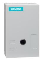
Electrically held lighting contactor, Contactor amp rating 20A, 0 N.C. / 3 N.O. Poles, 220VAC 50HZ/240VAC 60HZ coil, Non-combination type, (no disconnect device), Enclosure NEMA type 1, Indoor general purpose use
