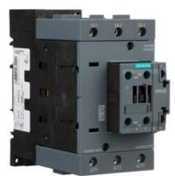
Electrically held lighting contactor, Contactor amp rating 100A, 0 N.C. / 3 N.O. Poles, 208VAC 50/60HZ coil, 1 NO / 1 NC auxiliary contacts Non-combination type, (no disconnect device), Enclosure NEMA type (open), No enclosure
