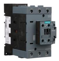
Electrically held lighting contactor, Contactor amp rating 100A, 0 N.C. / 3 N.O. Poles, 24VAC 50/60HZ coil, 1 NO / 1 NC auxiliary contacts Non-combination type, (no disconnect device), Enclosure NEMA type (open), No enclosure
