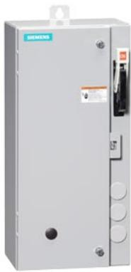
Electrically held lighting contactor, Contactor amp rating 30A, 0 N.C. / 3 N.O. Poles, 198VAC 50HZ/208VAC 60HZ coil, Combination type, 30A/600V non-fuse disconnect, Enclosure NEMA type 12, Dust/drip proof for indoors
