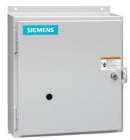
Electrically held lighting contactor, (convertible to mech. held), Amp rating 30A (tungsten 20A), 8 N.C. / 2 N.O. poles, 460-480V 60Hz/440V 50Hz coil, Noncombination type, Encl NEMA type 4X 304 S-Steel, Water/dust tight noncorrosive
