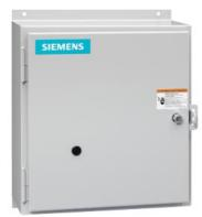
Electrically held lighting contactor, (convertible to mech. held), Amp rating 30A (tungsten 20A), 8 N.C. / 1 N.O. poles, 115-120V 60Hz/110V 50Hz coil, Non-combination type, Encl NEMA type 4X 304 S-Steel, Water/dust tight noncorrosive
