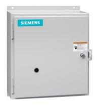
Electrically held lighting contactor, (convertible to mech. held), Amp rating 30A (tungsten 20A), 8 N.C. / 0 N.O. poles, 347V 60Hz coil, Non-combination type, Encl NEMA type 4X 304 S-Steel, Water/dust tight noncorrosive
