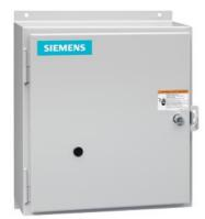
Electrically held lighting contactor, (convertible to mech. held), Amp rating 30A (tungsten 20A), 6 N.C. / 6 N.O. poles, 347V 60Hz coil, Non-combination type, Encl NEMA type 4X 304 S-Steel, Water/dust tight noncorrosive
