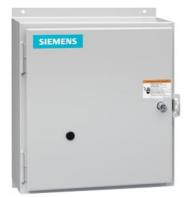
Electrically held lighting contactor, (convertible to mech. held), Amp rating 30A (tungsten 20A), 6 N.C. / 5 N.O. poles, 347V 60Hz coil, Non-combination type, Encl NEMA type 4X 304 S-Steel, Water/dust tight noncorrosive
