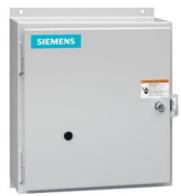
Electrically held lighting contactor, (convertible to mech. held), Amp rating 30A (tungsten 20A), 6 N.C. / 2 N.O. poles, 277V 60Hz / 240V 50Hz coil, Noncombination type, Encl NEMA type 4X 304 S-Steel, Water/dust tight noncorrosive
