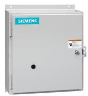
Electrically held lighting contactor, (convertible to mech. held), Amp rating 30A (tungsten 20A), 5 N.C. / 4 N.O. poles, 460-480V 60Hz/440V 50Hz coil, Noncombination type, Encl NEMA type 4X 304 S-Steel, Water/dust tight noncorrosive
