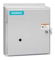
Electrically held lighting contactor, (convertible to mech. held), Amp rating 30A (tungsten 20A), 5 N.C. / 2 N.O. poles, 347V 60Hz coil, Non-combination type, Encl NEMA type 4X 304 S-Steel, Water/dust tight noncorrosive
