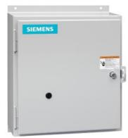
Electrically held lighting contactor, (convertible to mech. held), Amp rating 30A (tungsten 20A), 4 N.C. / 4 N.O. poles, 277V 60Hz / 240V 50Hz coil, Noncombination type, Encl NEMA type 4X 304 S-Steel, Water/dust tight noncorrosive
