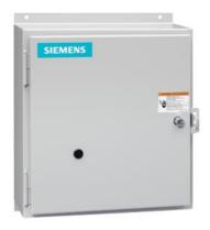
Electrically held lighting contactor, (convertible to mech. held), Amp rating 30A (tungsten 20A), 4 N.C. / 3 N.O. poles, 24V 60Hz / 20V 50Hz coil, Non-combination type, Encl NEMA type 4X 304 S-Steel, Water/dust tight noncorrosive
