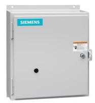
Electrically held lighting contactor, (convertible to mech. held), Amp rating 30A (tungsten 20A), 2 N.C. / 10 N.O. poles, 347V 60Hz coil, Non-combination type, Encl NEMA type 4X 304 S-Steel, Water/dust tight noncorrosive
