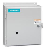
Electrically held lighting contactor, (convertible to mech. held), Amp rating 30A (tungsten 20A), 2 N.C. / 7 N.O. poles, 24V 60Hz / 20V 50Hz coil, Non-combination type, Encl NEMA type 4X 304 S-Steel, Water/dust tight noncorrosive
