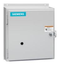
Electrically held lighting contactor, (convertible to mech. held), Amp rating 30A (tungsten 20A), 2 N.C. / 1 N.O. poles, 200-208V 60Hz coil, Non-combination type, Encl NEMA type 4X 304 S-Steel, Water/dust tight noncorrosive
