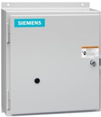
Electrically held lighting contactor, (convertible to mech. held), Amp rating 30A (tungsten 20A), 1 N.C. / 9 N.O. poles, 277V 60Hz / 240V 50Hz coil, Non-combination type, Encl NEMA type 4X 304 S-Steel, Water/dust tight noncorrosive
