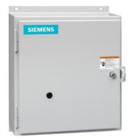
Electrically held lighting contactor, (convertible to mech. held), Amp rating 30A (tungsten 20A), 0 N.C. / 10 N.O. poles, 200-208V 60Hz coil, Non-combination type, Encl NEMA type 4X 304 S-Steel, Water/dust tight noncorrosive
